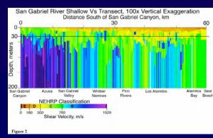
A 60-km long cross section of the upper 200 m of the Los Angeles basin, at 100X vertical exaggeration, showing shear-wave speed. The image was derived using seismic surface-wave background noise. (From W. Thelen et al., BSSA, 96, 1055, 2006)
