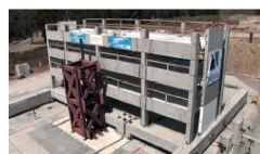
Half-scale parking structure on the NEES shake table at UCSD in 2008. Courtesy of UCSD Jacobs School of Engineering.
