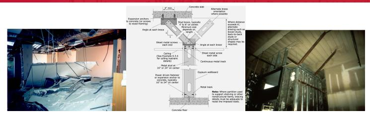
Photos and illustration from the light interior partition wall component example in FEMA E-74. Left photo (courtesy of Wiss, Janney, Elstner Associates) shows failure of inadequately braced partial height partitions in the 1994 Northridge earthquake. Center detail illustrates seismic mitigation solution for nonstructural, partial height stud wall. Photo on right (courtesy of Degenkolb Engineers) shows appropriately braced partial height stud partition.
