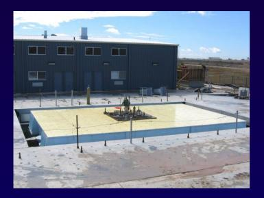
Platen 12.20 m x 7.6 m Max stroke 1.5 m Max velocity 1.8 m/sec Laminar soil box Two adjacent soil pits
