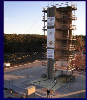
7-story reinforced concrete building test at UCSD NEES outdoor shake table showed that a structural wall with half the amount of reinforcing steel required by most building codes, but with more optimal layout, can better resist seismic loads. (Test funded by industry consortium) (Photo courtesy of Jose Restrepo, UCSD)
